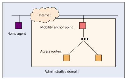
Figure 3. *Hierarchical architecture.*
