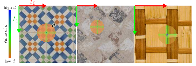
Figure 10: Distance function d applied around the local minimum of d (corresponding to ground truth period vectors of \mathbf{t}_0 and \mathbf{t}_1 ) on various textures. d was only evaluated with orthogonal period vectors to produce this visualization.
