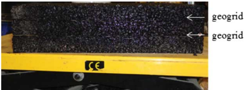
Figure 5. Three-layered asphalt slab, reinforced with two geogrids.
