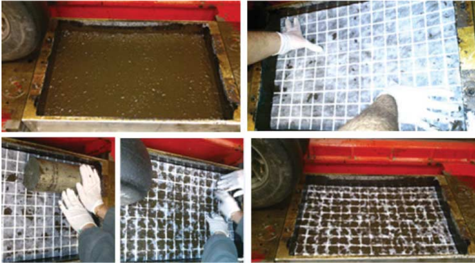
Figure 4. Insertion and installation of the geogrid on the bitumen emulsion layer.
